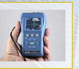
Danatronics introduces the first ever hand held ultrasonic precision thickness gages with COLOR A-Scan. The UPG-O7DLCW is a hand held ultrasonic precision thickness gage designed to non-destructively measure most engineering materials with the greatest thickness range. So if you are measuring coil steel, fiberglass thickness on boats, titanium golf club heads, plastic bottles or even rubber tires . . . put us to test, we measure up.
